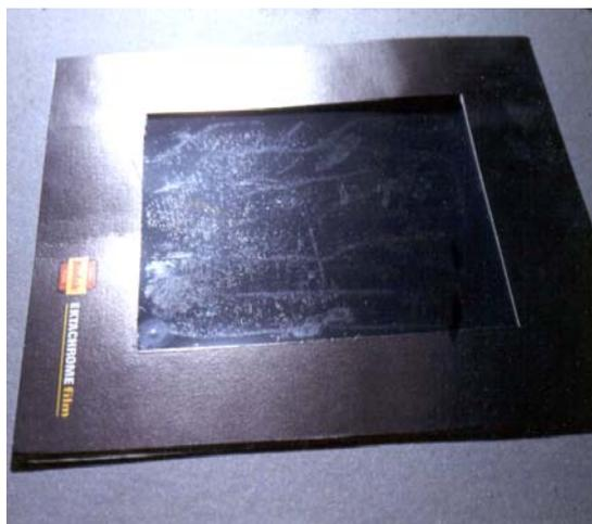
*Figure 4.12 Crystals of phthalic acid deposited on photographic positive from PVC photograph pocket*
