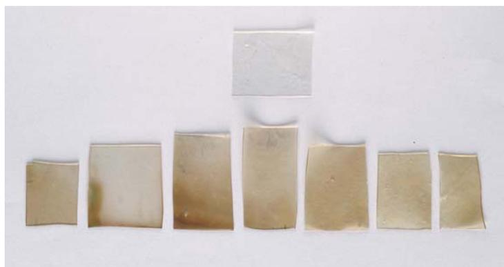
*Figure 6.12 Solvay model sheets before (upper sample) and after thermal ageing with silica gel. Discolouration is uneven and greatest at the lower edge of all sheets, that closest to the silica gel during ageing.*
