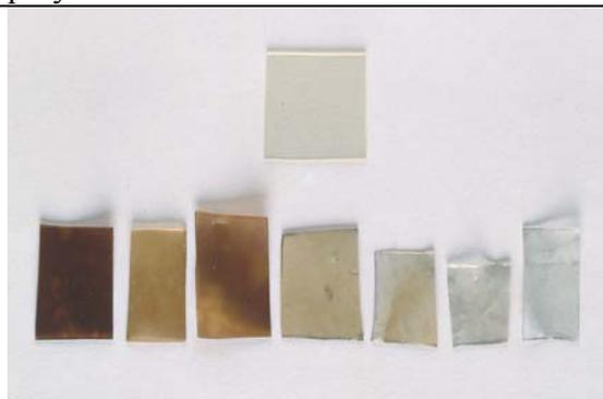
*Figure 6.14 Solvay model sheets before (upper sample) and after thermal ageing with activated carbon for 65 days. Sheets containing least plasticizer were most discoloured. Carbon particles adhered to the tacky surfaces of more highly plasticized sheets.*
