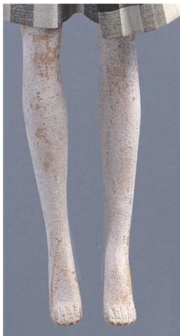
*Figure 4.14 Doll's legs showing a high concentration of stearic acid crystals on surface*
