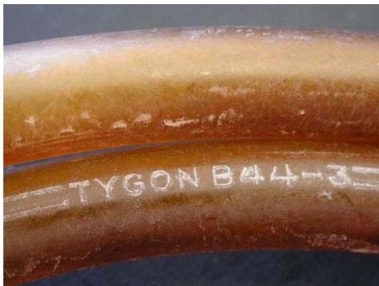
*Figure 4.8 Yellowed life support tubing from Apollo space suit showing crystalline phthalic acid on inner and outer surfaces. The tube is 15mm in diameter*
