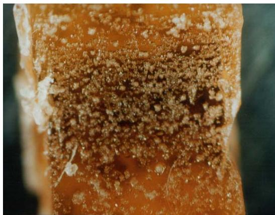
*Figure 4.9 Crystals on inside surface of life support tube*
