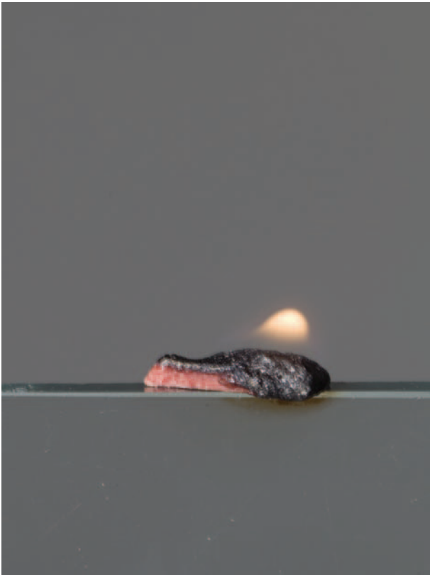
Figure 5.10 Flame test with melamine-formaldehyde. Expands and chars on burning.
