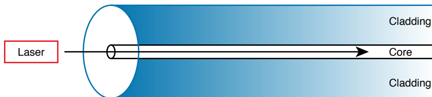
Figure 2-17 Transmission on Single-Mode Fiber with Laser Transmitter
