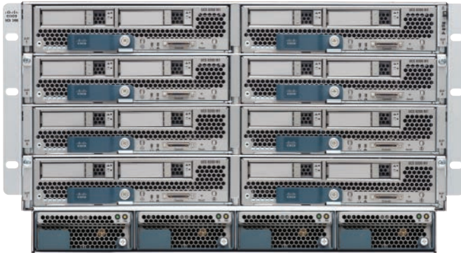
Figure 15-1 Cisco UCS Servers: B-Series (Blade)
