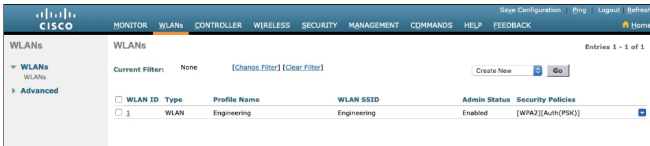
Figure 29-20 Displaying WLANs Configured on a Controller
