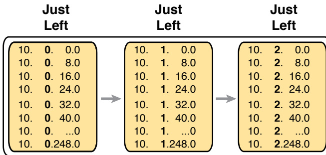
Figure M-2 Creating Subnet Blocks by Adding 1 in the “Just Left” Octet
