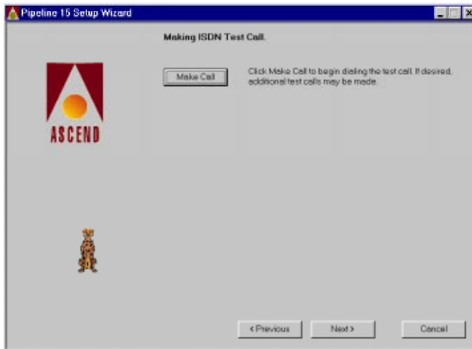
When you click Make Call, depending on the calling mode, one or two of the B-channel lights on the front of the Pipeline go on. Then the transmit data (tx) light goes on momentarily. The test can take up to 90 seconds. A dialog will tell you if the test was successful or not.
