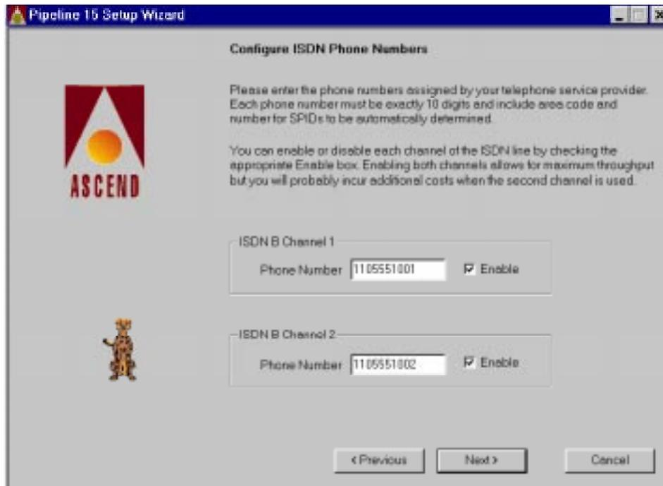
Enter the phone numbers and enable the line(s) you want the Pipeline to use for data calls. You can make and receive voice calls even if a data call is in progress, so you can enable both lines for data and still use all the voice features of the Pipeline. See the section on Voice calls to see how the Pipeline handles voice calls.
