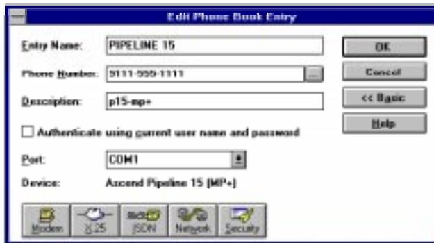
Supply an Entry name, phone number, and description. If you click “Authenticate using current user name and password,” the uses your Windows NT sign-on user name and password. Be sure the COM port setting is correct.
