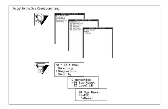
To restart your Multiband VSX using the Sys Reset command:
