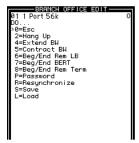
In the Do menu, press ctrl - N until the cursor reaches R=Resynchronize, and press enter.
