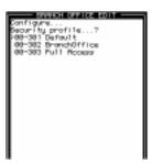
4 If necessary, press ctrl - N to move the cursor to the Security profile you want to activate. Then press enter to select it.
