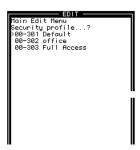
If necessary, press ctrl - N to move the cursor to the Security profile you want to activate. Then press enter to select it.
