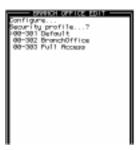
If necessary, press ctrl - N to move the cursor to the Security profile you want to select. Then press enter to select it.
