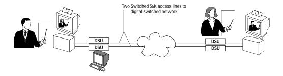
Using two ISDN B channels to aggregate 112-128kbps:
