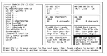
A thick black border appears around the 00-100 status window, indicating that it is active. You can scroll through the window to view additional information about your Multiband VSX's system.
