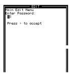
In the brackets, type the password for the profile you want to activate. Then press enter to accept it.
