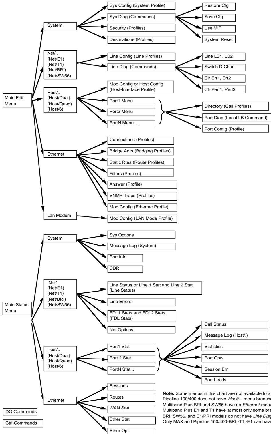
The preceding illustration shows the names and relative locations of Multiband Plus-BRI menus, commands, and profiles.
