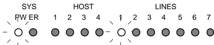
Figure 5: Front Panel LEDs, D-Channel of Line 1 Active
