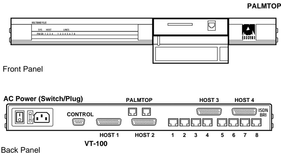
Figure 2: Front and Back Panels of Multiband Plus-BRI
