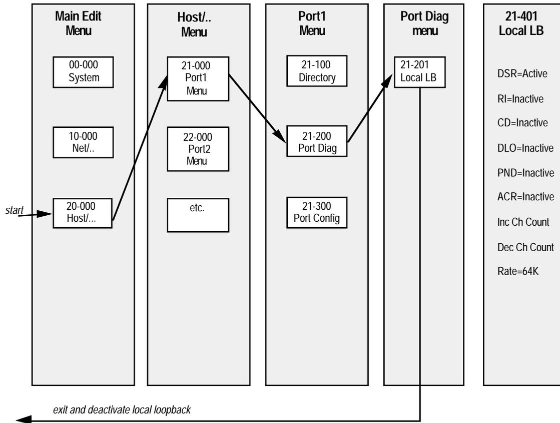
Figure 7: Sequence of steps to activate local loopback
