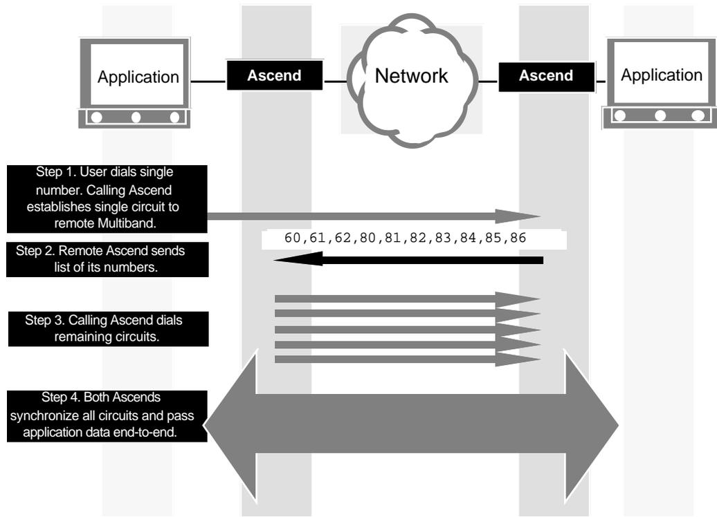
AIM and BONDING calls are established using the following steps:
