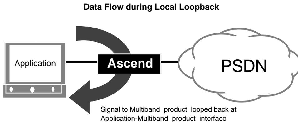
You can terminate the loopback test at any time by exiting the Local Loop submenu with the **Left-Arrow** key. When you end a local loopback test, all of the control leads revert to the state they were in before the test was begun.
