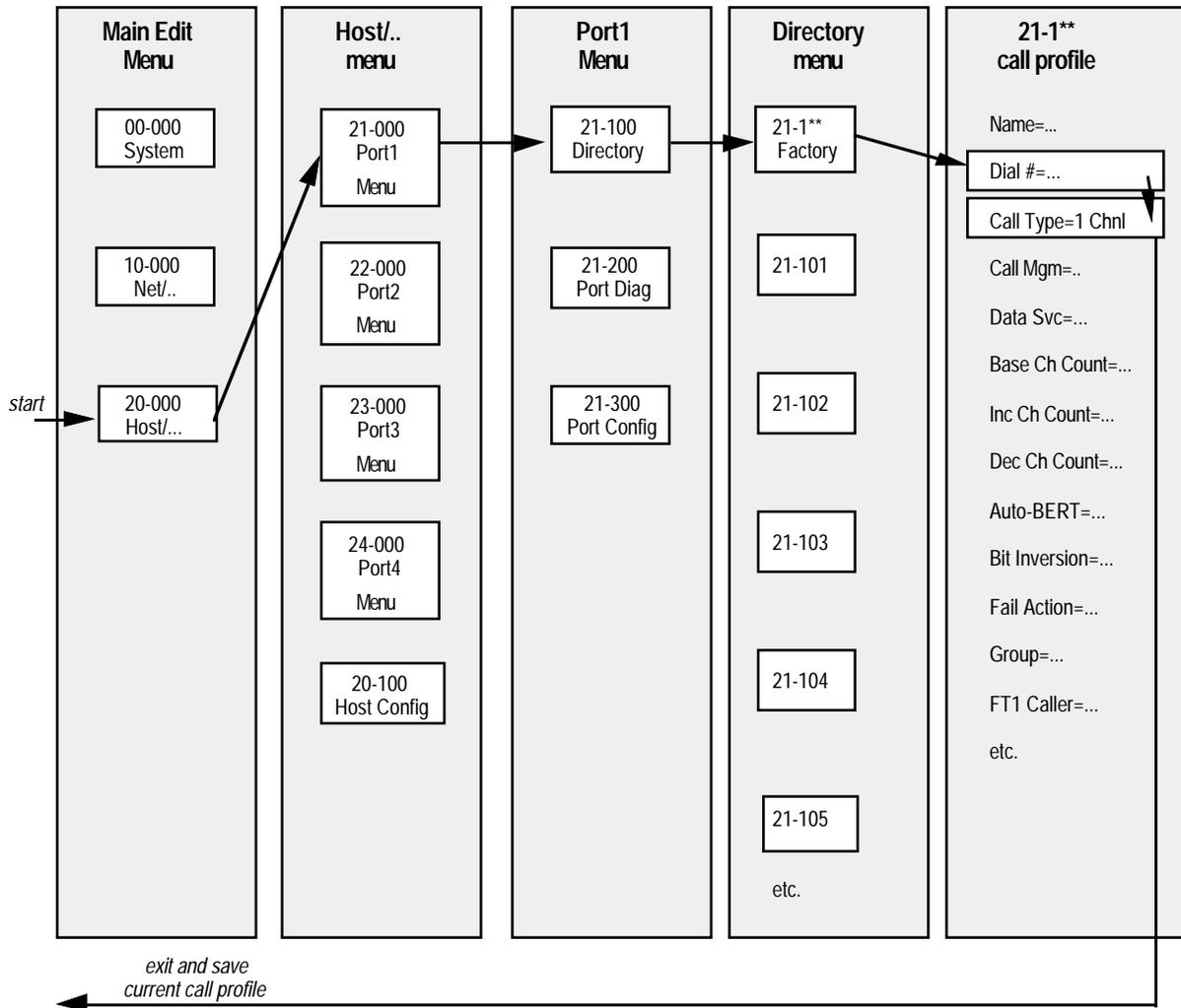
Figure 6: Configuration of Current Call Profile of Host Port #1 for Test Call
