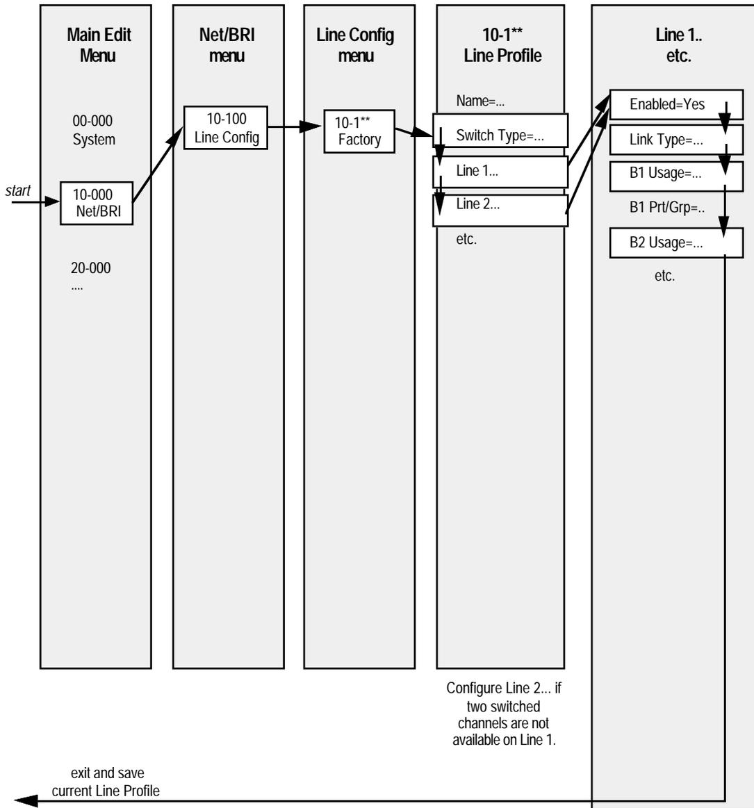
Figure 4: The parameters involved in configuring your BRI interface
