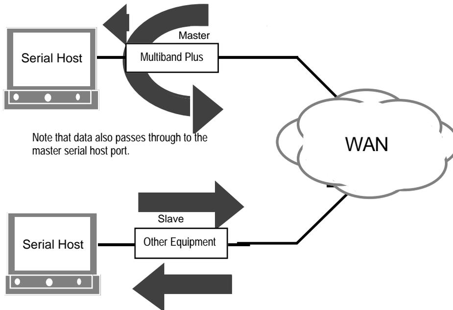
2. Slave transmits data toward the master Multiband Plus which loops it back toward the slave.
