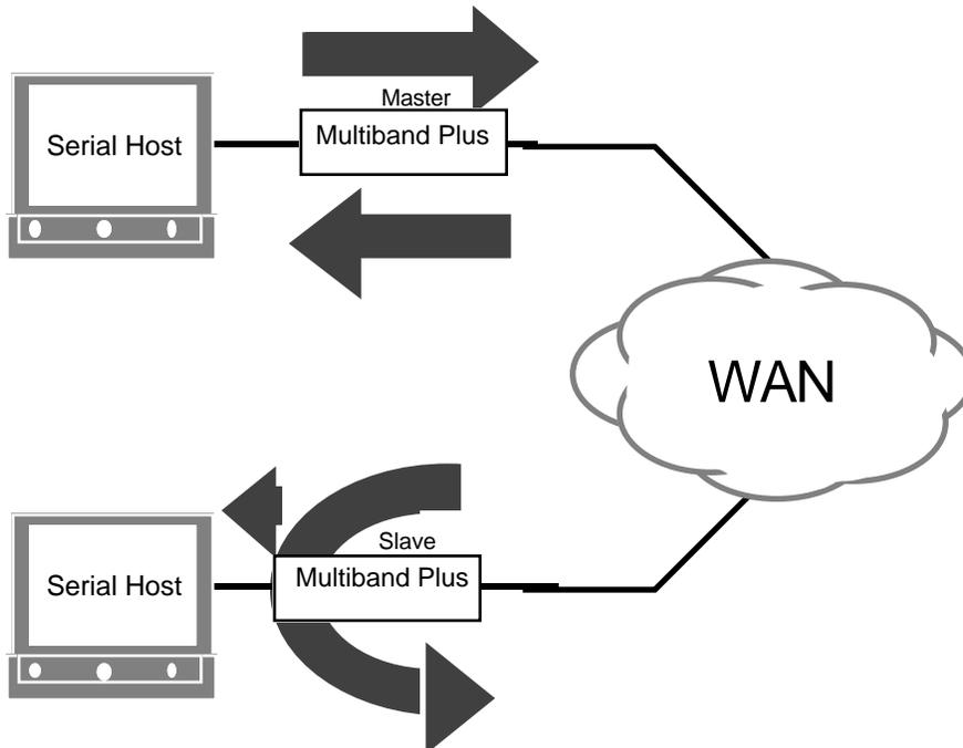
2. ...and data loops at the slave serial host interface toward master Multiband Plus.
