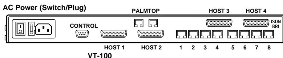
Figure 8: Back Panel of Multiband Plus
