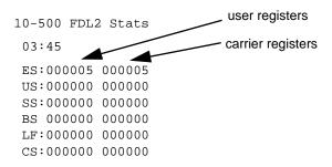
You can reset the user performance registers using Clr Perf1 and Clr Perf2 in the Line Diag menu, but only the carrier can reset the carrier registers. All performance registers are reset upon power-up or software reset.
