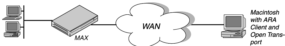
Figure 3-7. An ARA connection enabling IP access
