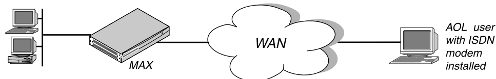
Figure 3-9. A TCP-clear connection
