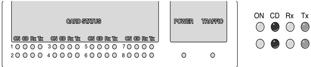
Figure 2-6. PC card Status LEDs
