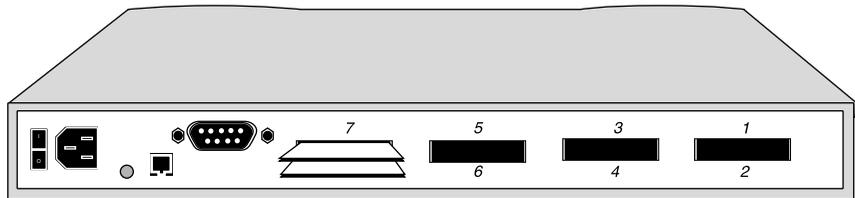
*Figure C -1. MAX 200Plus back panel with vertical slot numbering*
