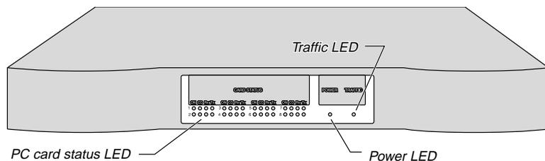
Figure 2-2. MAX 200Plus front panel
