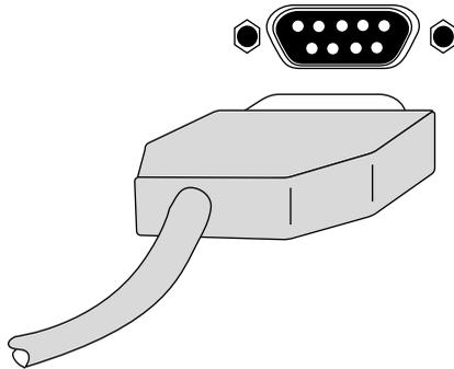
*Figure 2-5. Connecting to Thick Ethernet*
