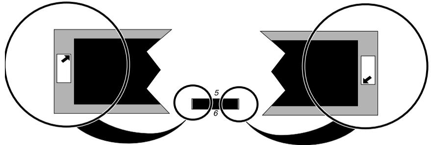
Figure 2-4. PC card eject buttons
