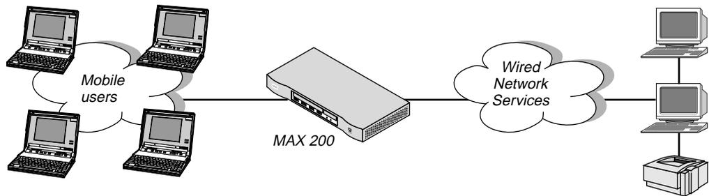
Figure 1-1. A remote access switch gives mobile users access to wired network services
