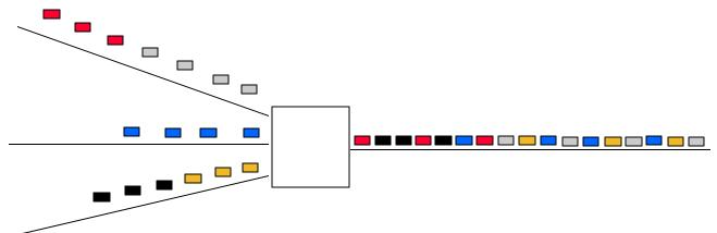
IP Navigator solves this problem by merging VPs, using the VCI to identify each source within the VP
