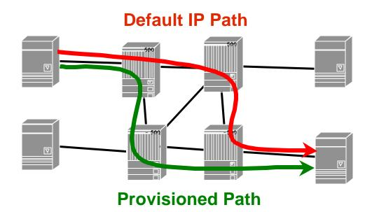
Provision a different route than IP routing would use to override routing and efficiently utilize bandwidth
