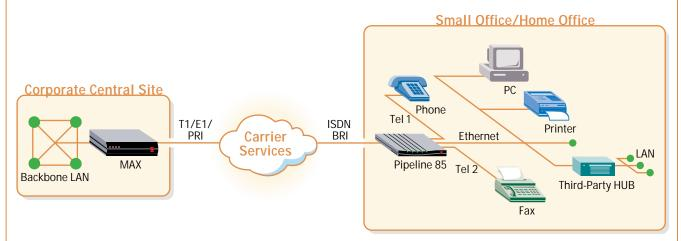
The Pipeline 85 makes it easy to connect multiple users to a corporate central site. If more than four connections are required, additional hubs can be "daisy-chained" from the Pipeline 85 to support up to 1,024 users.
