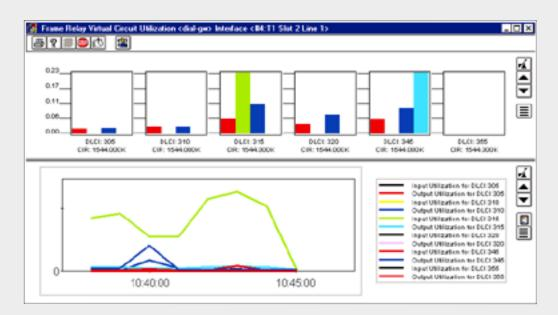
NavisAccess offers network managers detailed information about the network. This view shows the Frame Relay Virtual Circuit Utilization for a five minute interval.
