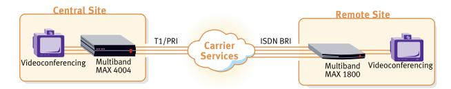
Multiband MAX users leverage the existing switched network by utilizing bandwidth on demand technology and the Ascend Inverse Multiplexer (AIM) to support cost-effective, bandwidth-intensive videoconferences between two or more sites. Bandwidth sessions can range from 56 Kbps to 4 Mbps.
