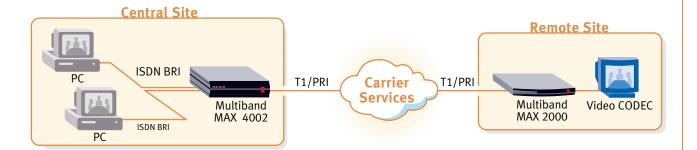
ISDN signaling supports ISDN connections straight to the desktop for digital services dial-in traffic that utilizes multimedia applications requiring voice, video and data.
