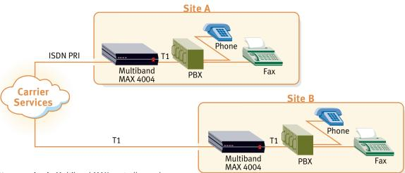
PRI to T1 conversion in Multiband MAX controllers enhances networking options while assuring maximum use of T1 capability. Excess circuits from the PRI network can be passed to a T1 circuit for use by a PBX for voice.
