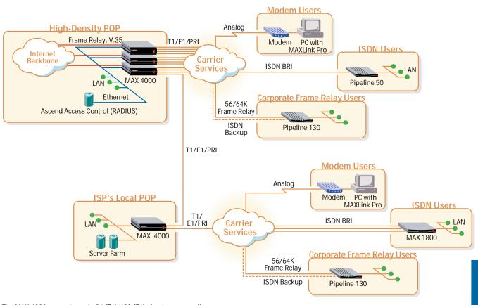
The MAX 4000 supports up to 96 (T1)/120 (E1) simultaneous calls from ISDN BRI, Frame Relay or modem users to the backbone network over ISDN PRI, channelized T1/E1 or ISDN BRI lines. Up to 72 of the 96 (T1)/120 (E1) calls can be from modem users.
