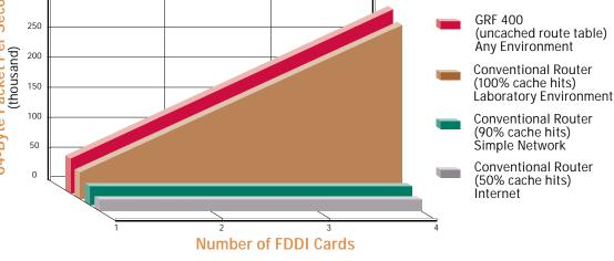
Conventional router performance degrades rapidly when placed in networks that route traffic to a large number of IP addresses. In these networks, routers using caches treat most IP addresses as new addresses, forcing them to perform a software-based, full route table lookup. Even with 50 percent cache hits, a conventional router's aggregate packet-per-second performance plummets to less than 4 percent of a fully-configured GRF 400.
