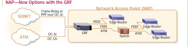
The GRF is the ideal solution for growing a NAP environment. It fits easily into existing topologies and offers cost-effective design options for expanding the network. Support for new media types such as OC-12c, Frame Relay or PPP over SONET OC-3c provides new options for NAP designs.
