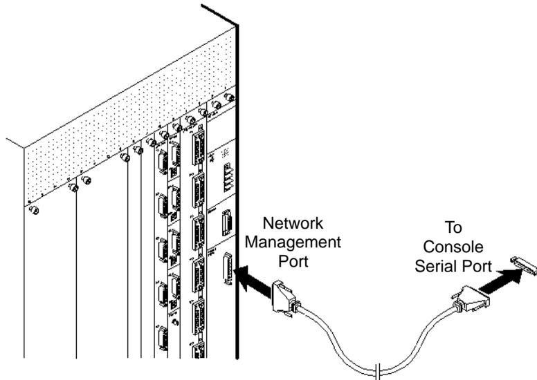
**Figure 4-3. Console Connection to B-STDX Switch**
