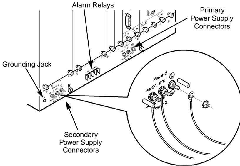
**Figure 6-8. Connecting the -48 VDC Power Supply**
