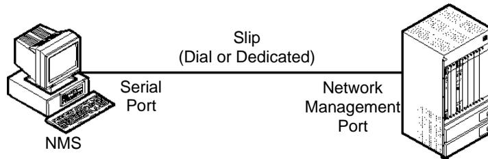
Figure 4-6. Serial Line Over Internet Protocol (SLIP) Method
