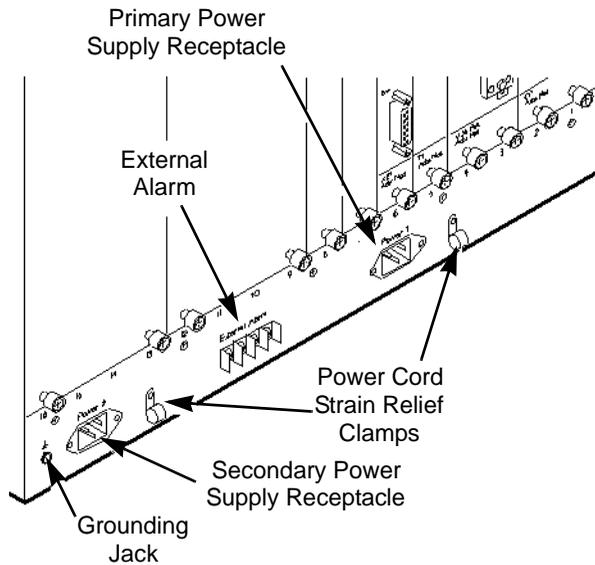
**Figure 6-5. AC Power Supply Module Back View**
