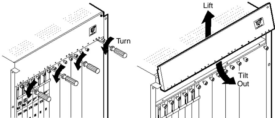
**Figure 6-9. Removing the Cooling Fan Access Cover**
