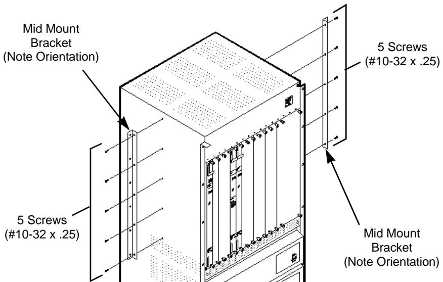
**Figure 4-2. Installing Mid-Mount Brackets**
