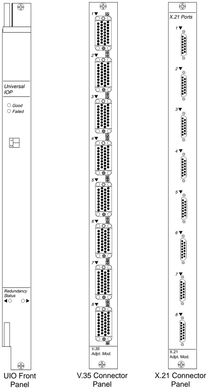
**Figure A-1. 8-Port UIO Module, V.35 Panel, and X.21 Panel**
