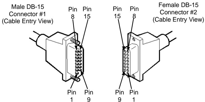
**Figure B-7. X.21 Straight-through Cable Diagram**
