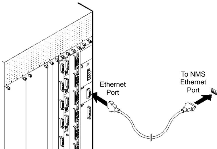
**Figure 4-8. Direct Ethernet Connection from B-STDX Switch to NMS**
