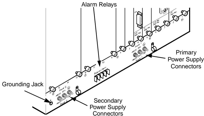
**Figure 6-6. -48 VDC Power Supply Module Back View**
