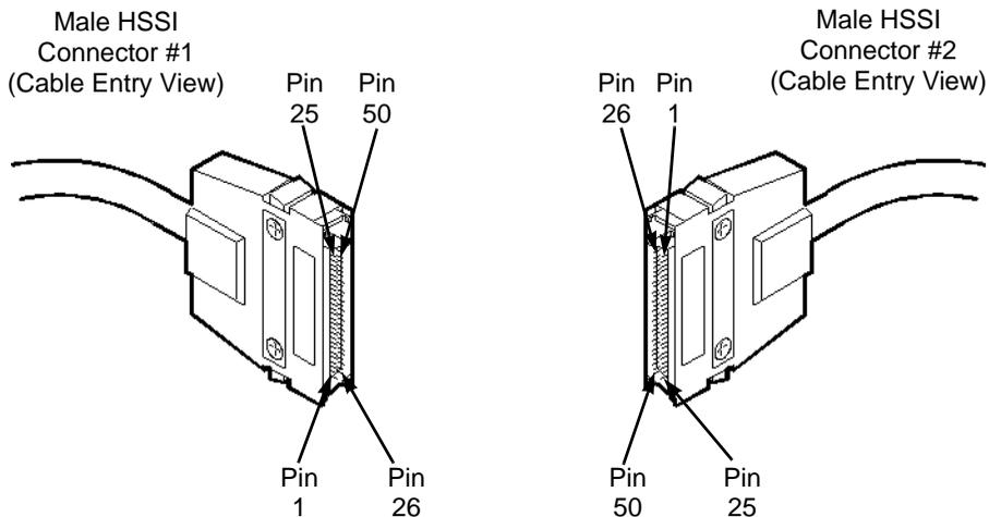
**Figure B-13. HSSI Straight-through Cable Diagram**
