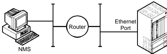
Figure 4-5. Indirect Ethernet Method
