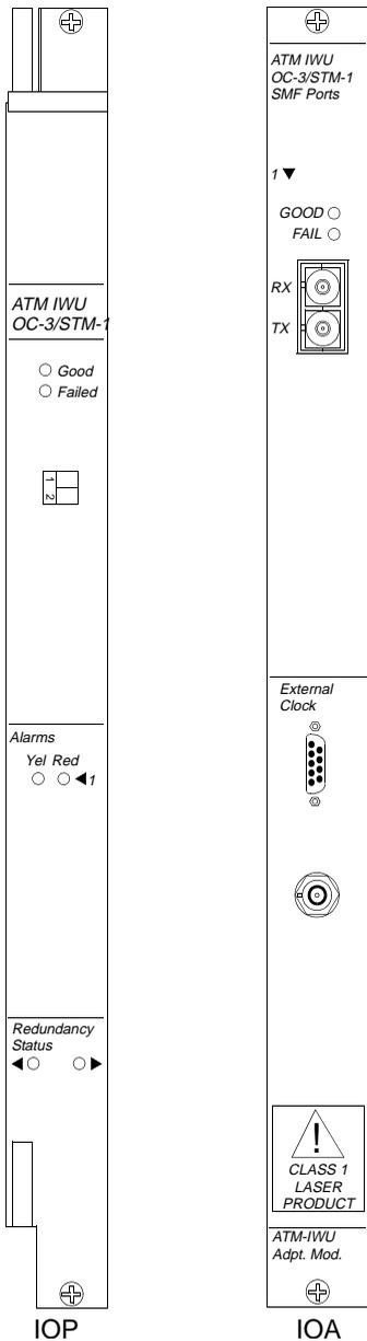
**Figure A-14. ATM IWU OC-3c/STM-1 IOP and IOA**
