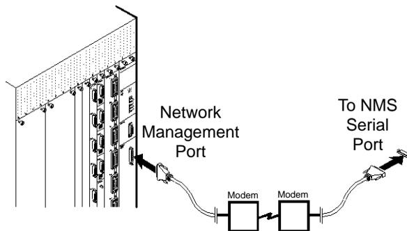
**Figure 4-11. Dial SLIP Connection from B-STDX Switch to NMS**
