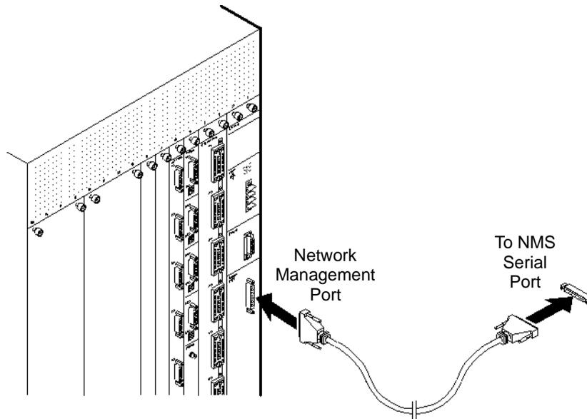
**Figure 4-10. Sample Direct SLIP Connection from B-STDX Switch to NMS**
