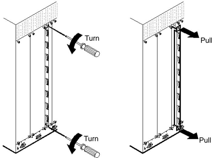
**Figure 6-4. Removing IOA Modules**
