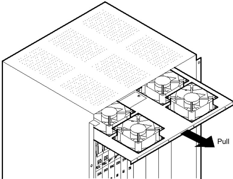
**Figure 6-10. Removing the Cooling Fan Module**
