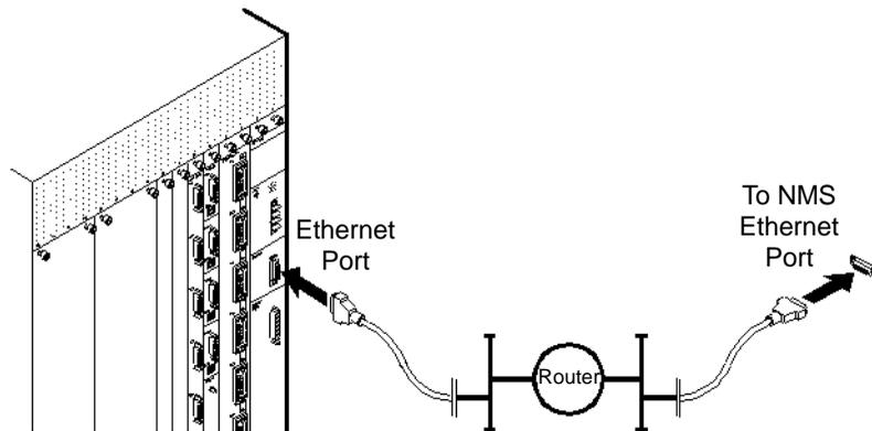
**Figure 4-9. Indirect Ethernet Connection from B-STDX Switch to NMS**
