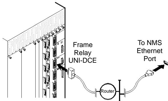
**Figure 4-12. Management DLCI Connection from B-STDX Switch to NMS**
