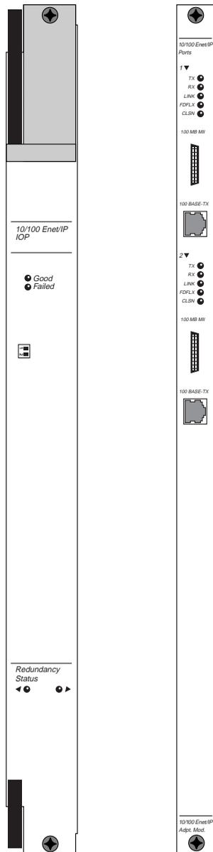
Figure A-15. Ethernet 10/100Base-T IOP and IOA
