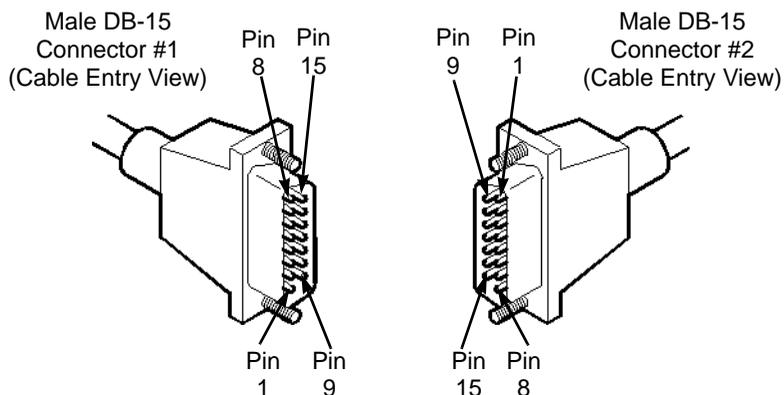
**Figure B-9. T1/E1 Straight-through Cable Diagram**
