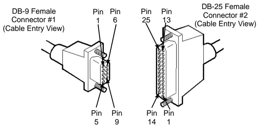
**Figure B-4. RS-232 DB-9 to DB-25 Shielded Crossover Cable Diagram**
