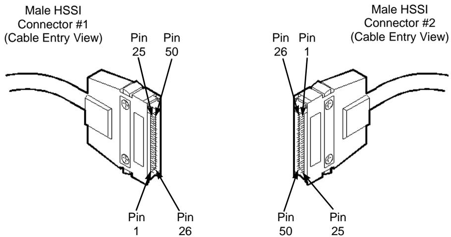
**Figure B-14. HSSI Crossover Cable Diagram**
