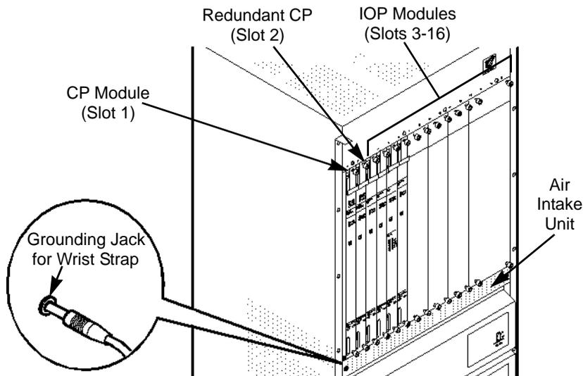
**Figure 3-2. Front View of the B-STDX 9000**
