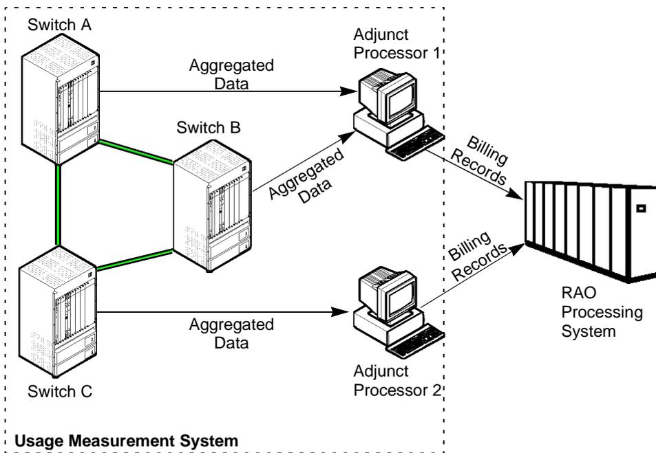
**Figure 1-2. Sample Billing System Hardware Configuration**
