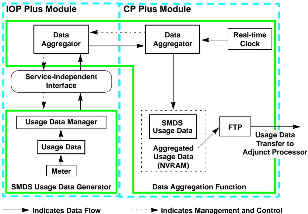
**Figure 2-1. B-STDX Billing System Components**
