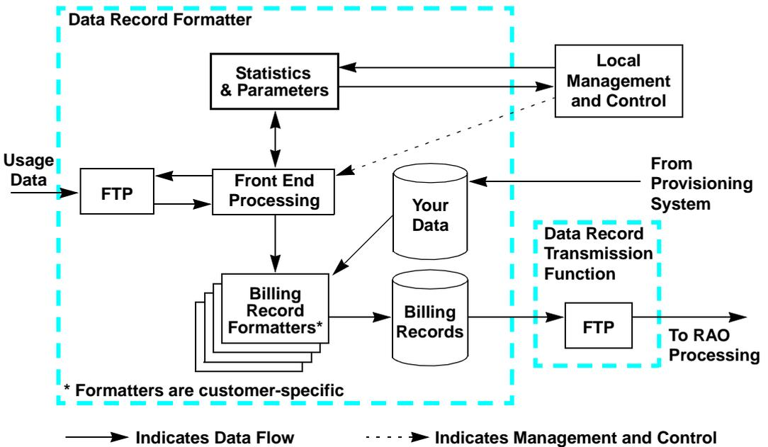
**Figure 2-2. Adjunct Processor Billing System Components**
