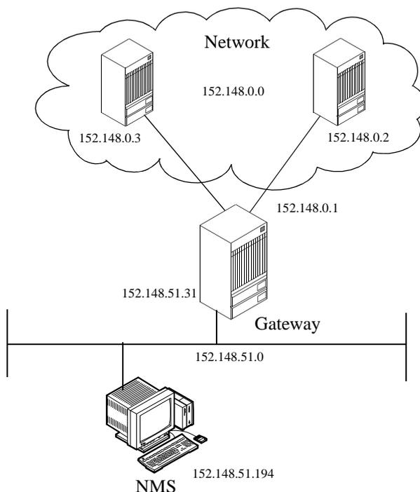
**Figure 7-5. Static Route Connection Example**
