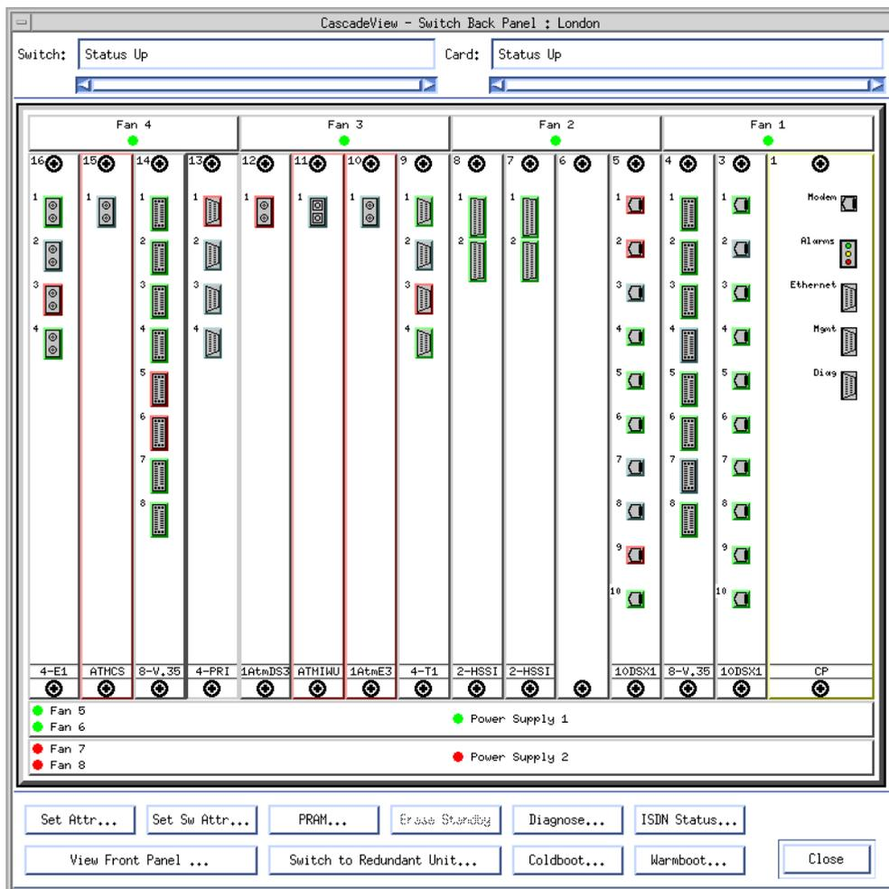
**Figure 6-1. Switch Back Panel Dialog Box**
