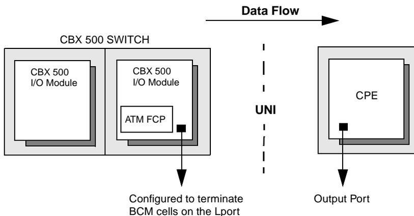
**Figure 2-5. Output UNI Logical Port RM Termination**
