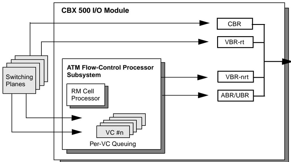
**Figure 2-1. CBX 500 Queues and the ATM Flow-Control Processor**
