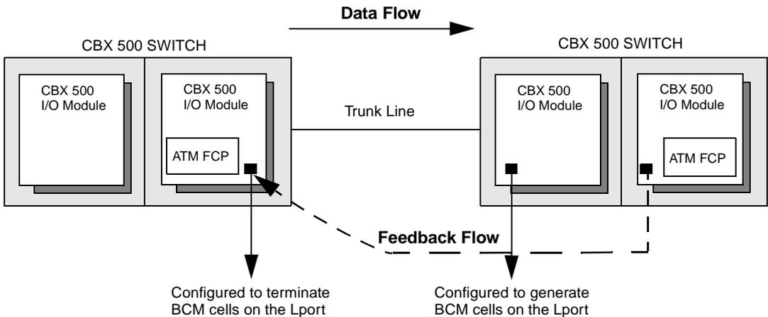
**Figure 2-4. BCM Closed-Loop Flow Control**
