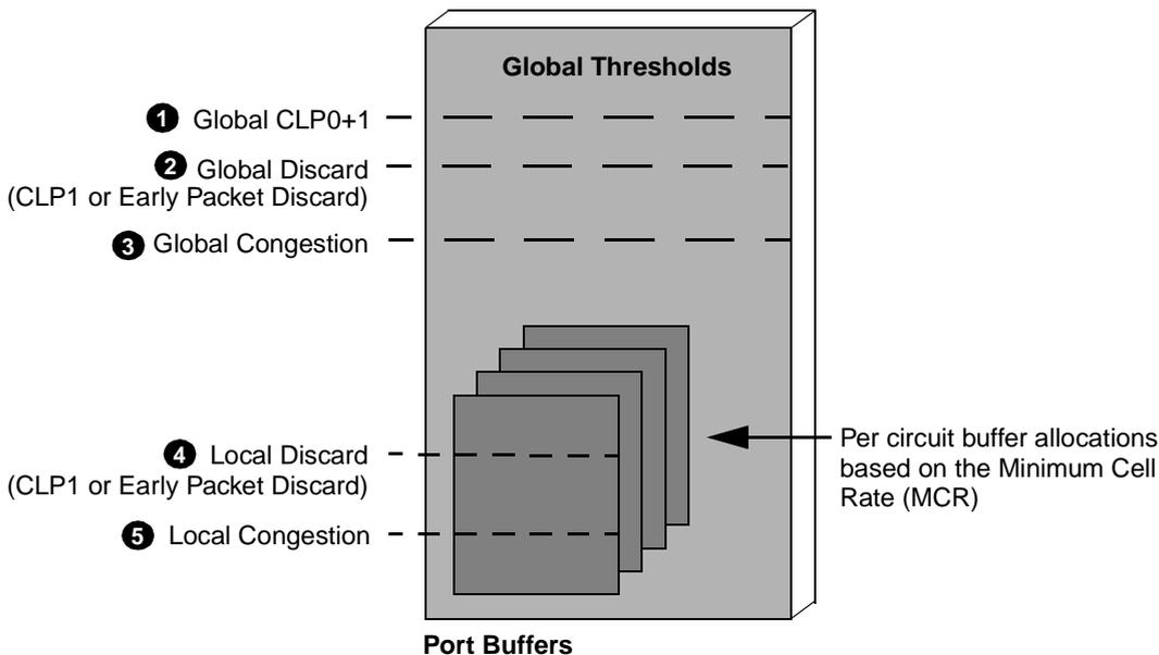
**Figure 2-6. ATM Flow-Control Processor Buffers**
