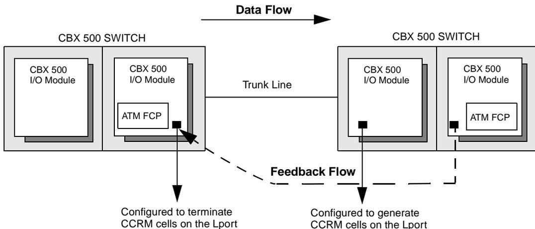
**Figure 2-3. CCRM Closed-Loop Flow Control**
