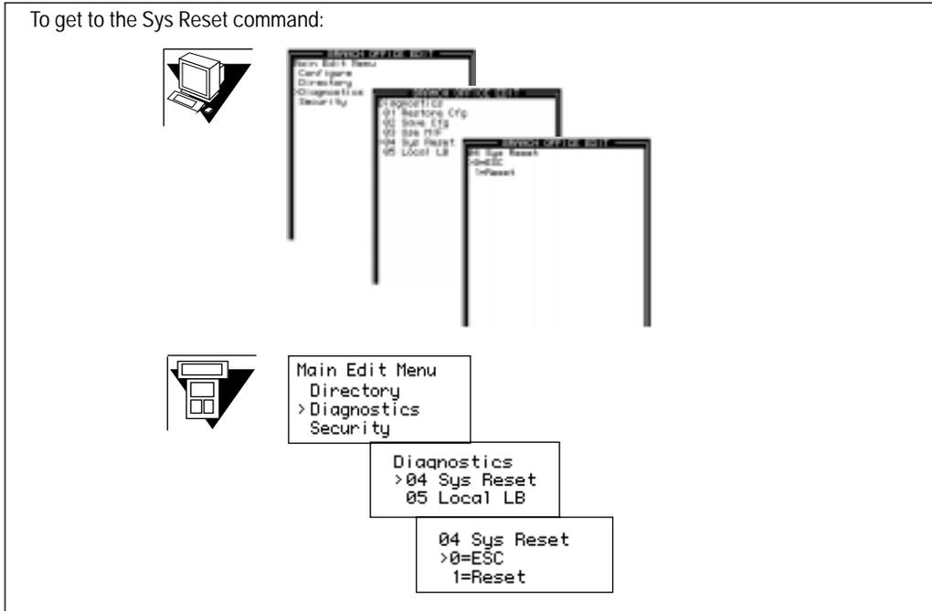
To restart your Multiband VSX using the Sys Reset command:
