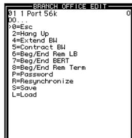
**3 In the Do menu, press **ctrl-N** until the cursor reaches R=Resynchronize, and press **enter**.**
