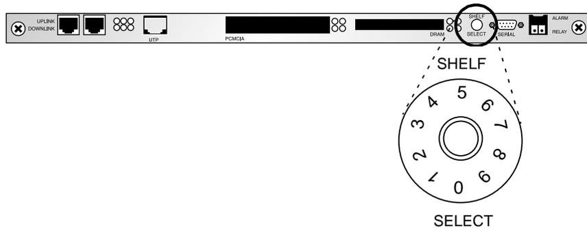
Figure 4-1. Setting the rotary switch to a unique number
