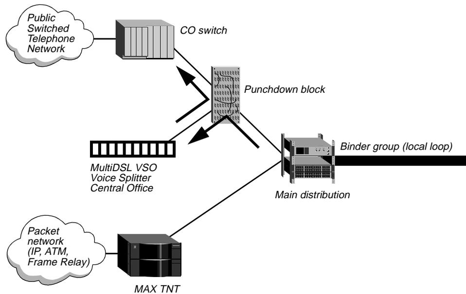
Figure B-1. Example of central office ADSL voice splitter set up
