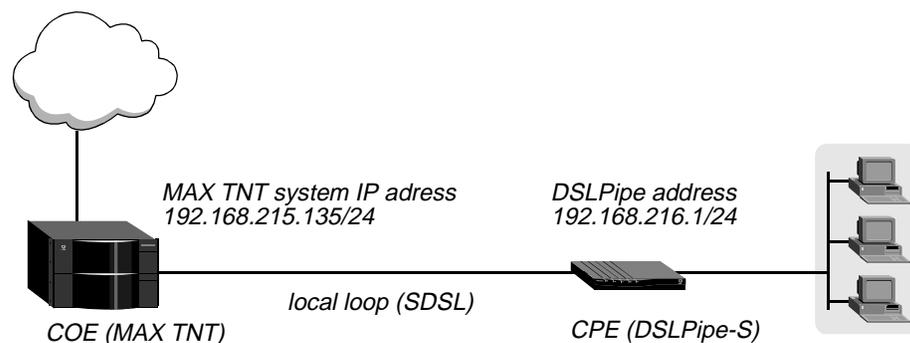
Figure 16-6. Example SDSL setup with system-based routing
