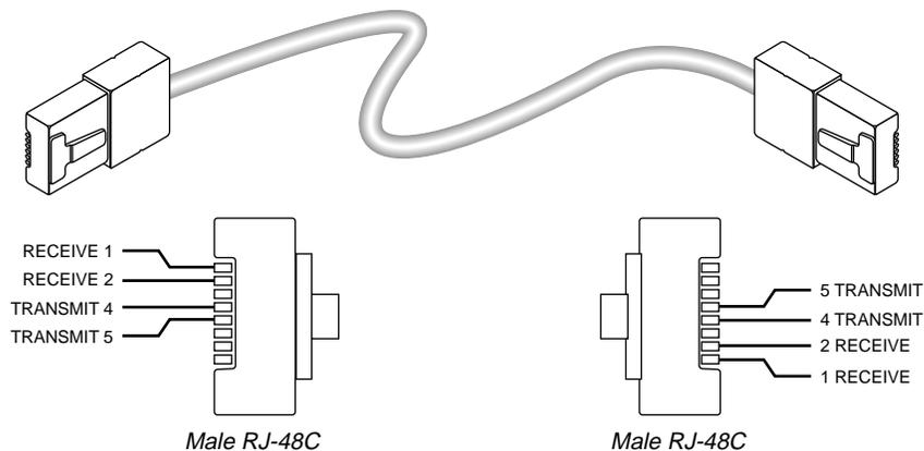
*Figure D-1. RJ-48C/RJ-48C crossover cable.*
