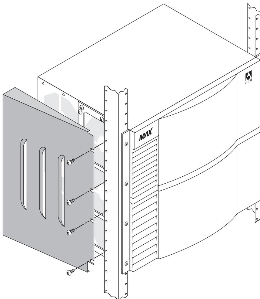
Figure 2-10. Exhaust shield installed in a cabinet
