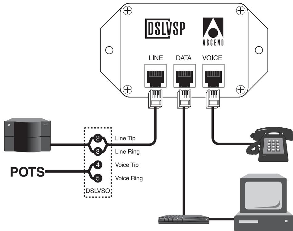
Figure B-5. Example of ADSL voice splitter wiring
