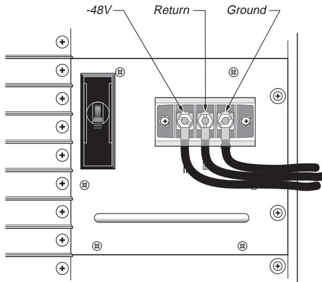
Figure 2-19. Connecting to dc power
