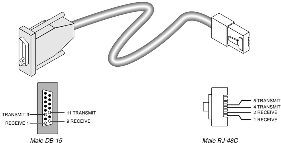
*Figure D-3. RJ-48C/DB-15 straight-through cable*
