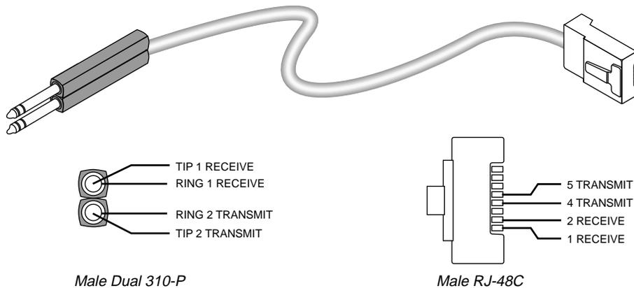
Figure D-5. RJ-48C/Bantam straight-through cable
