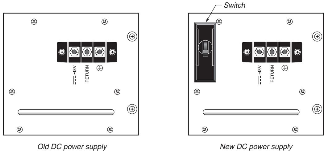
Figure 2-14. Identifying the high-output dc power supply
