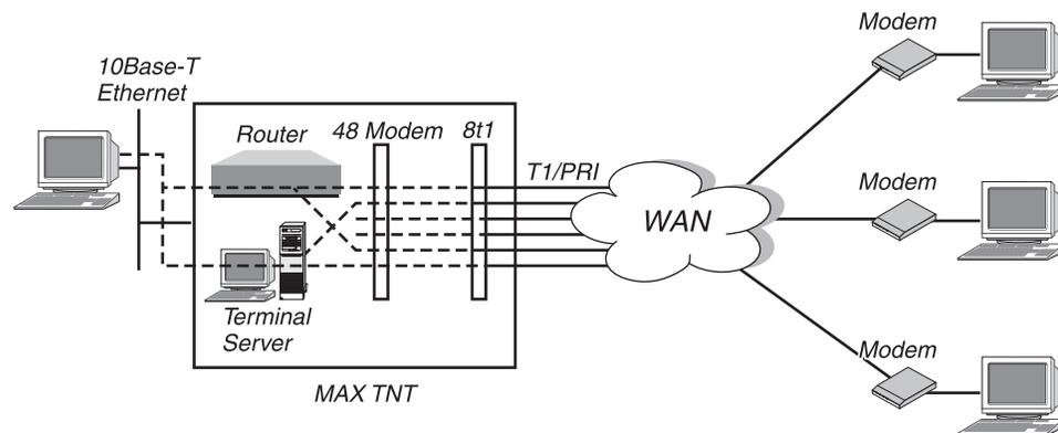
Figure 17-2. Routing inbound calls to a digital modem
