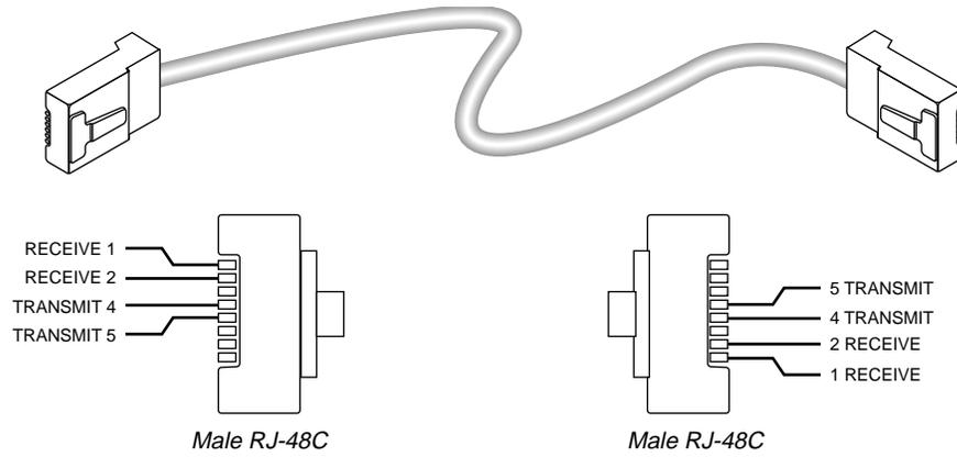
Figure D-2. RJ-48C/RJ-48C straight-through cable specifications
