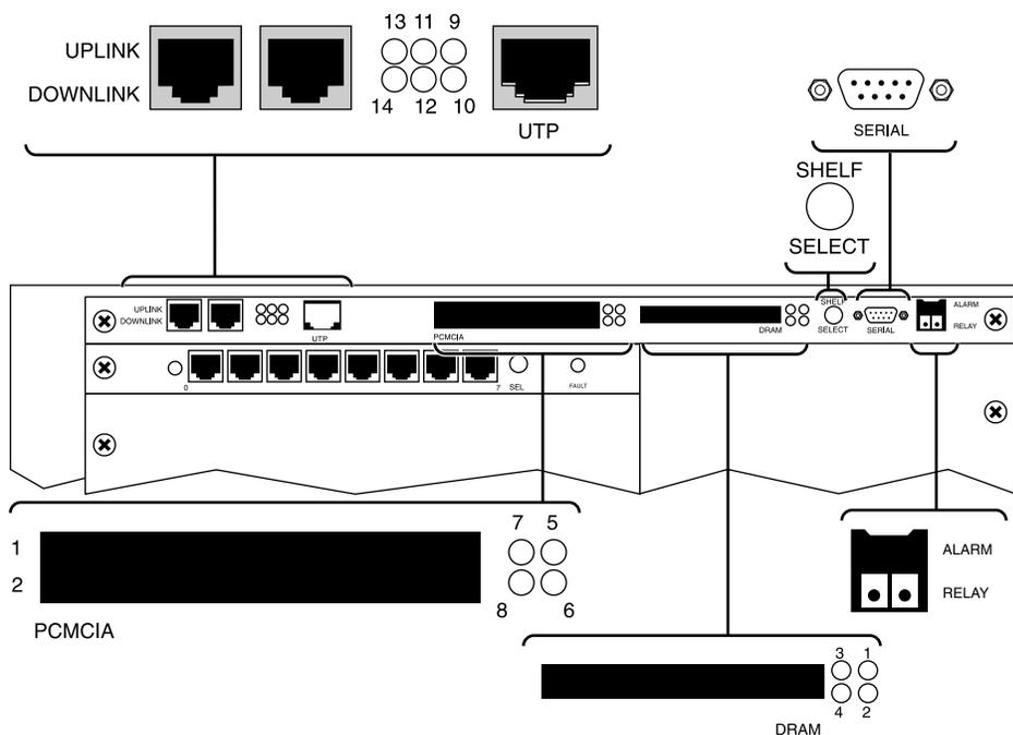
Figure 2-3. MAX TNT shelf-controller back panel
