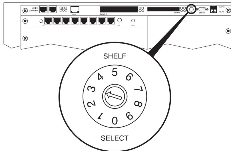
Figure 2-5. Verifying the rotary switch setting
