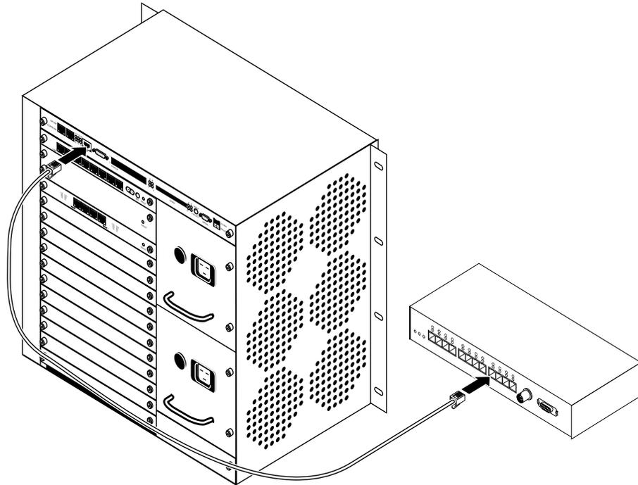
Figure 2-20. Connecting Ethernet cable
