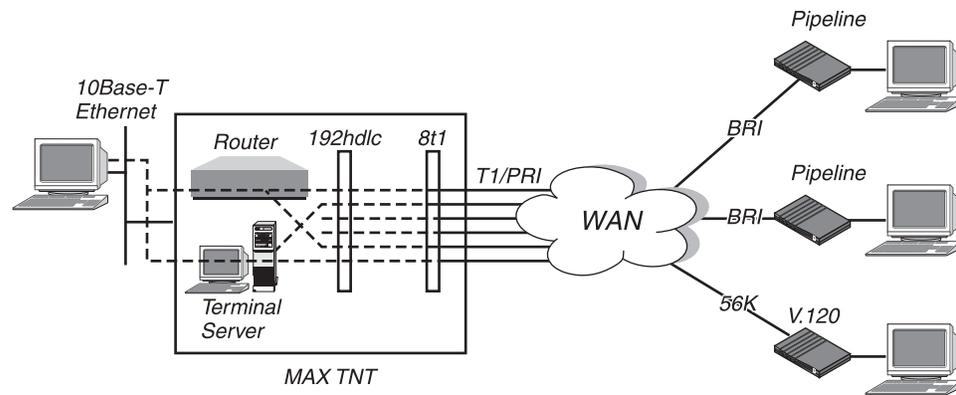
Figure 17-1. Routing inbound calls to an HDLC channel
