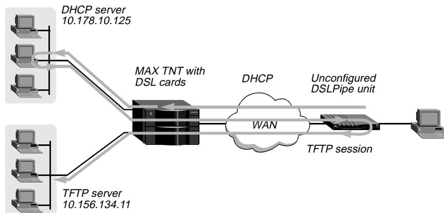
*Figure 16-1. DSLPipe unit obtaining its configuration (Plug & Play)*
