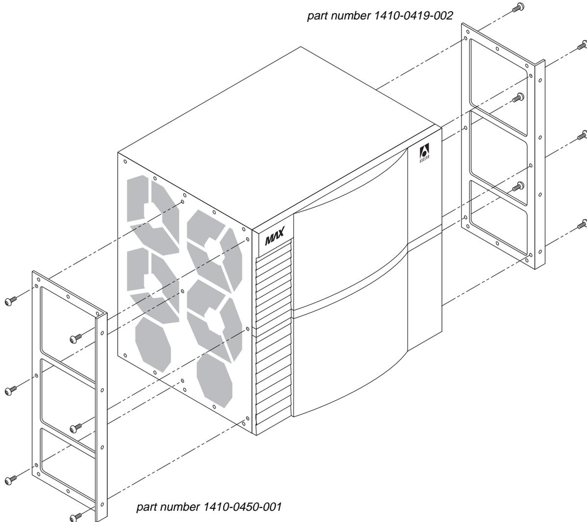
Figure 2-6. Installing the MAX TNT rack ears
