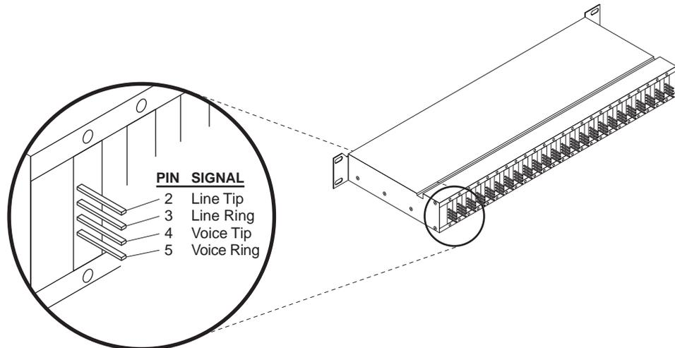
Figure B-4. DSLVS0 rack pins
