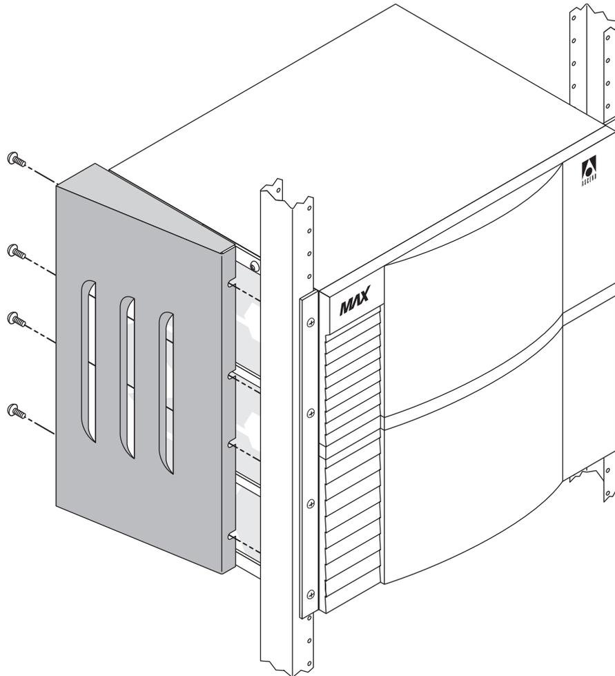
*Figure 2-9. Exhaust shield installed in a rack*
