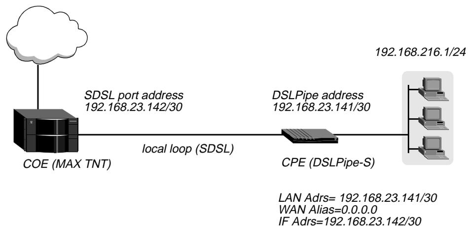
Figure 16-5. Example SDSL setup with interface-based routing
