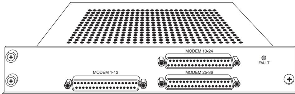
Figure 6-3. Analog Modem card
