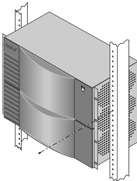
*Figure 2-8. Mounting the MAX TNT in a rack*
