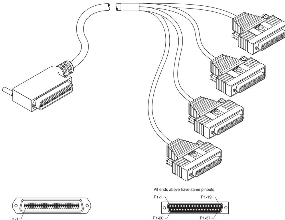
Figure D-8. ADSL 50-pin telco to quad DB-37 cable
