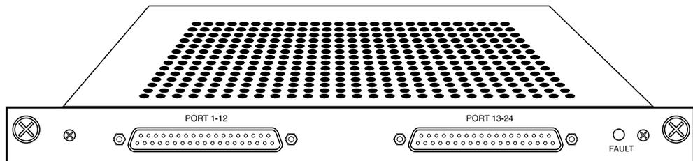
Figure 12-4. MAX TNT SDSL card
