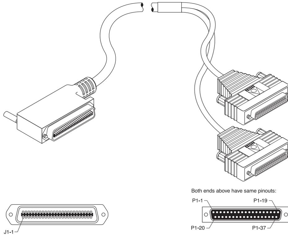
*Figure D-9. SDSL 50-pin telco to dual DB-37 cable*
