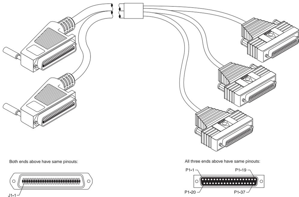
*Figure D-7. IDSL dual 50-pin telco to triple DB-37 cable*
