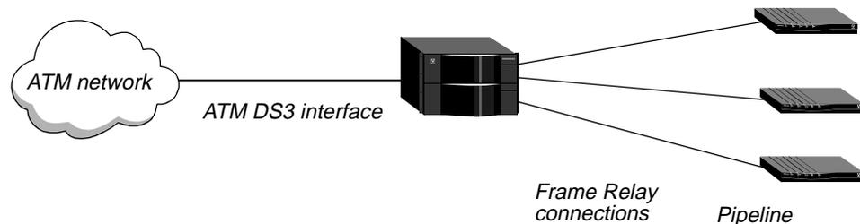
*Figure 13-5. Switched ATM-Frame Relay connection*
