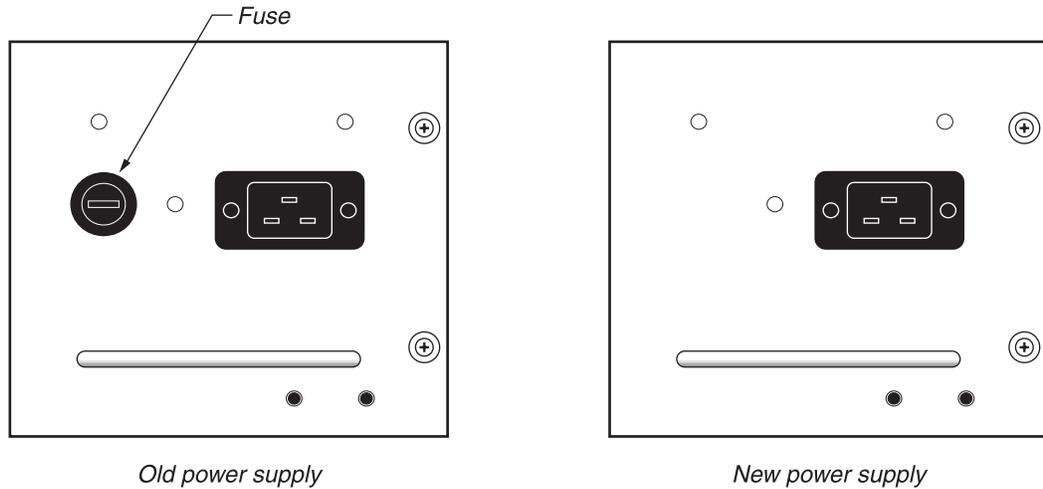
Figure 2-13. Identifying the high-output ac power supply
