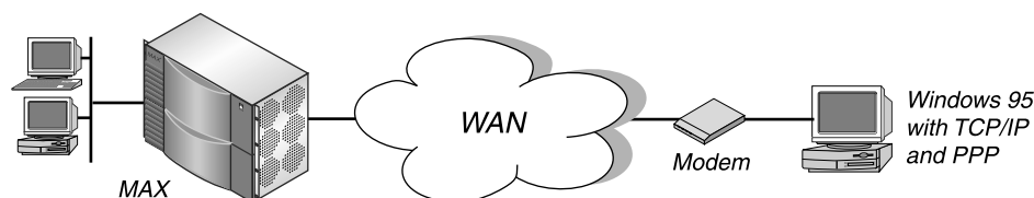
Figure 4-1. A PPP connection
