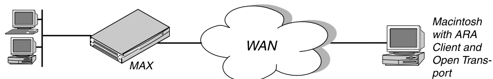
Figure 3-11. An ARA connection enabling IP access
