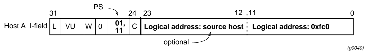
Figure 7-14. I-field for HIPPI-HIPPI IP routing example
